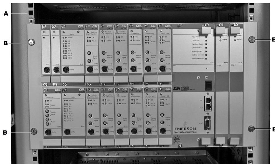
Figure 4-4: CSI 6500 mounted in a 19 in. cabinet enclosure
