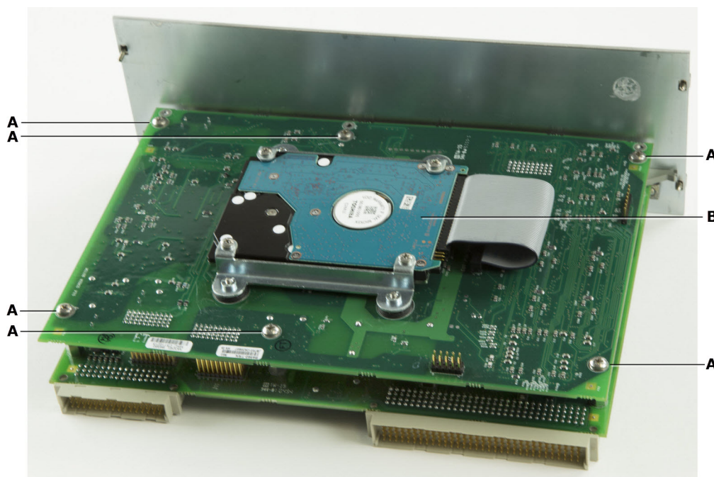
Figure 7-2: Transient Daughterboard PCB mounted on Processor module
