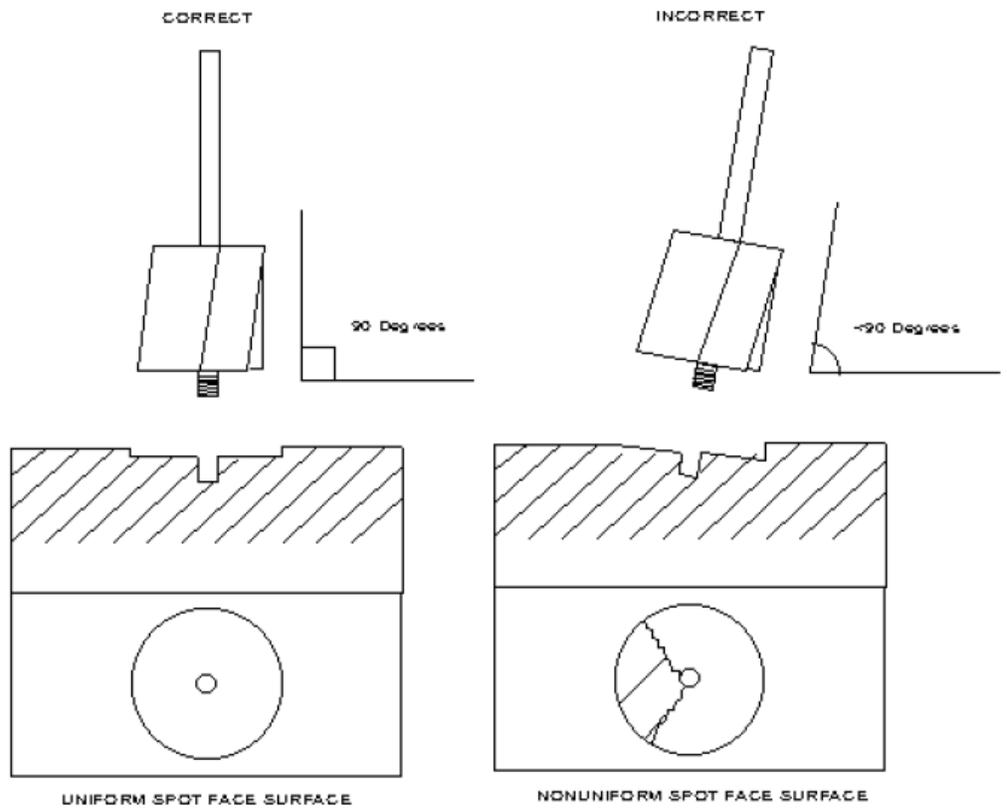
**Figure 4-10: Milling process for sensor mounting**
