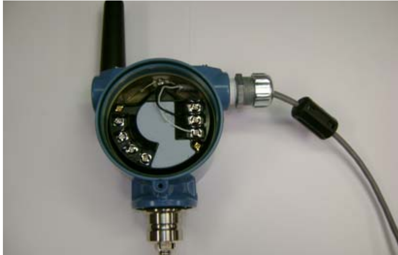
Figure D-10. Transmitter (CSI 9420), external power option, with ferrite, after installation
