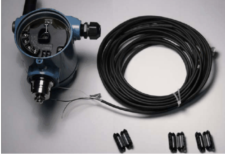
Figure D-6. Transmitter (CSI 9420), accelerometer with standard cable longer than 3 meters, and ferrites, pre-installation
