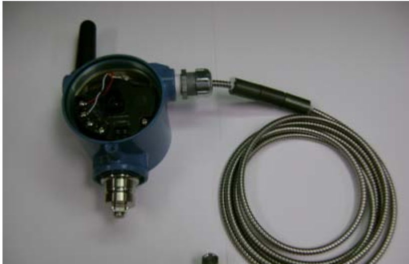
Figure D-9. Transmitter (CSI 9420), accelerometer with armor-jacketed cable, and ferrites, after installation
