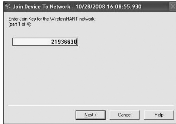
Figure 2-16. Join Device to Network screen: Join Key 1
