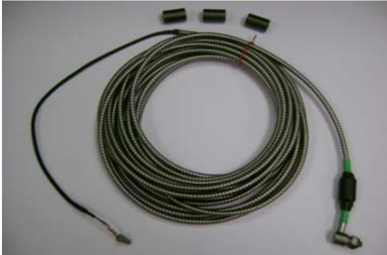
Figure D-8. Transmitter (CSI 9420), accelerometer with armor-jacketed cable, and ferrites, pre-installation
