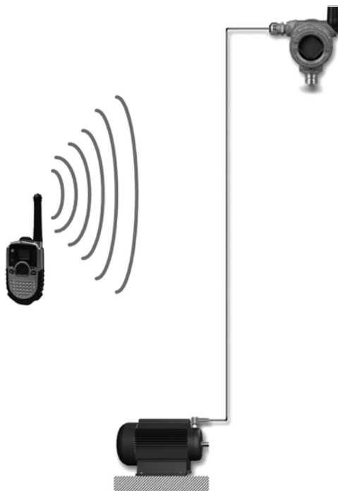
Figure D-12. RFI source polarization coincident with long cable run results in maximum interference
