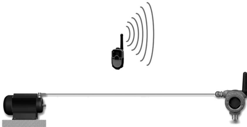
Figure D-11. RFI source cross-polarized with long cable run results in minimum interference
