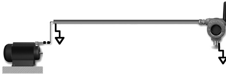
Figure D-2. Illustration of grounded conduit for added RFI protection
