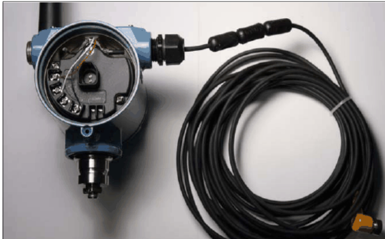
Figure D-7. Transmitter (CSI 9420), accelerometer with standard cable longer than 3 meters, and ferrites, after installation
