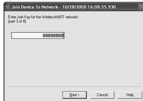
Figure 2-18. Join Device to Network screen: Join Key 3
