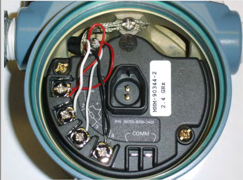
Figure 2: CSI 9420 wiring with two accelerometers
