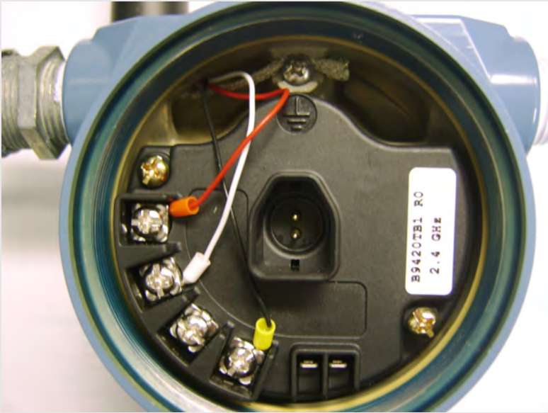
Figure 1: CSI 9420 wiring with one accelerometer
